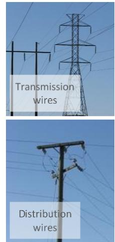
Source: Dominion. “Comparison of Transmission and Distribution Lines.” <http://bit.ly/220DfP0>. Accessed March 9, 2016.
